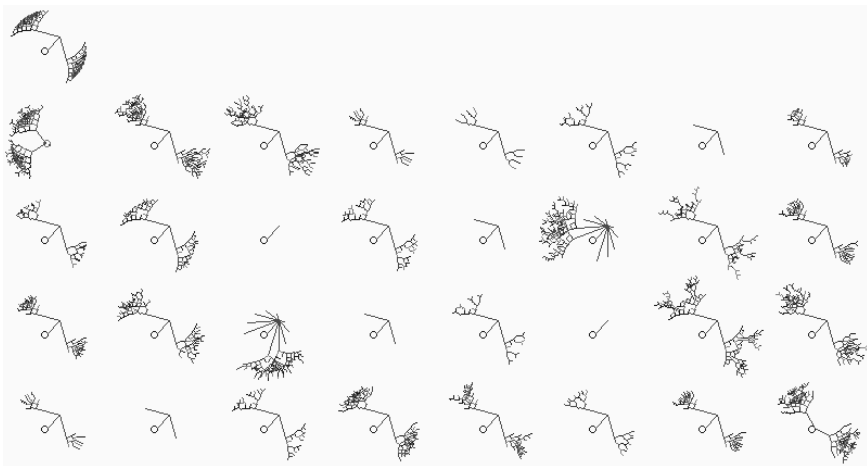
Fig. 11.25. Thirty-two mutant basins of attraction of the v=2 , k=3 rule 195 ( n=8 , seed all 0s). Top left: The original rule, where all states fall into just one very regular basin. The rule was first transformed to its equivalent k=5 rule (f00ff00f in hex), with 32 bits in its rule table for finer mutations. All 32 one-bit mutant basins are shown. If the rule is the genotype, the basin of attraction can be seen as the phenotype.
